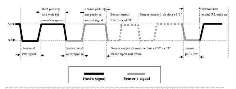
1) Step 1: MCU send out start signal to AM2302 and AM2302 send response signal to MCU
